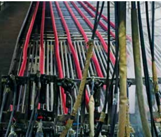
hoses during vulcanizing process
