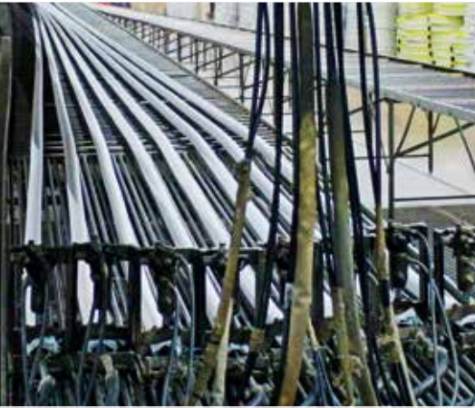
hoses during vulcanizing process
