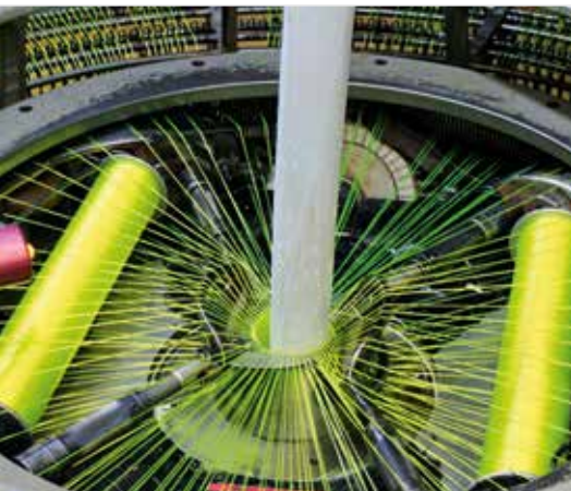
weaving process of jacket with incoming rubberlining
