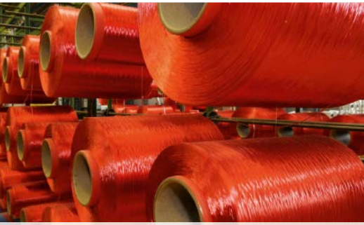
thread spools are plugged on the holding devices and will be used for twisting of warp and weft depending on jacket construction
