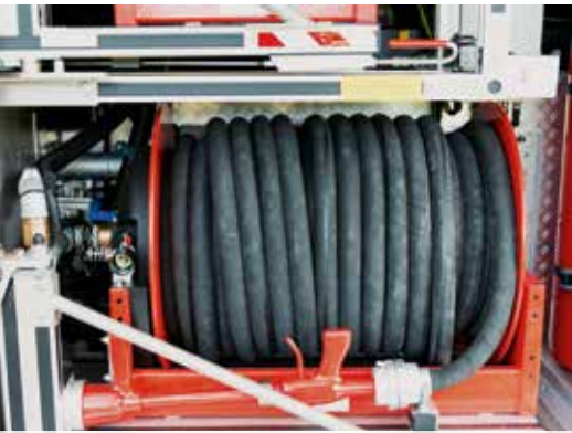
semi-rigid quick attack booster hose on reel in fire truck
